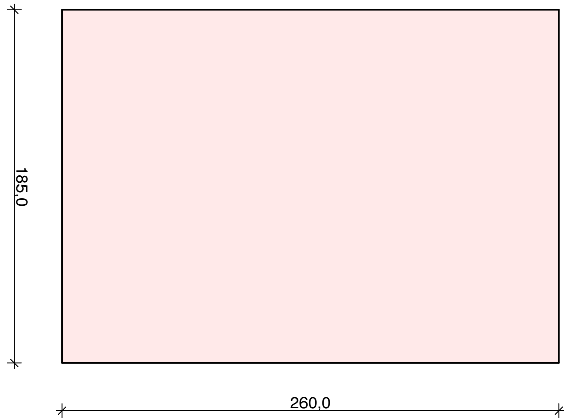
Pos_2.1 2 Pieces Sheet Metal 5 mm
